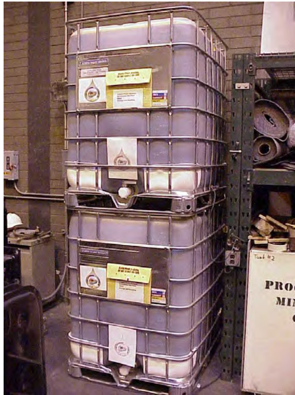
Figure 3: Example of 330 gallon tanks that ester fluid is delivered in.
